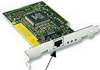
Ethernet Card – usually has only one jack.
